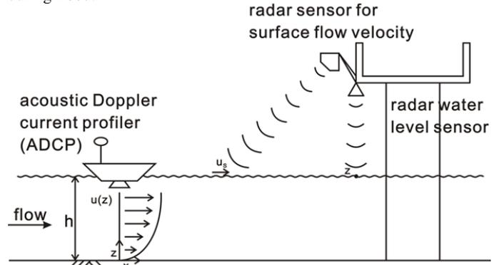
Fig. 3 Sensor and instrument arrangements for discharge measurements
