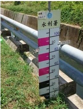
Fig. 6 Staff gauge for flooding depth measurement
