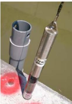
Fig. 7 Pressure-type sensor for flooding depth measurement
